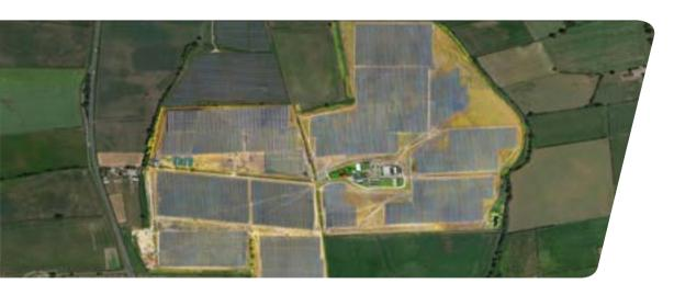
UK renewables developer GRIDSERVE has completed a "game changing" hybrid solar-plus-storage farm in York, unveiling a 34.7MW solar farm that boasts bifacial panels and single-axis trackers, a first for the UK solar market and what is thought to be the most northerly combination of the two cutting edge technologies in the world, bifacial panels and trackers and the site 'stacks' a number of revenue streams in order to be financially feasible without subsidy support.
